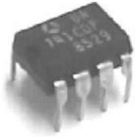
Figure 6: A picture of \mu\text{A741} operational amplifier (Left) and schematic of top view for pin assignment (Right)
