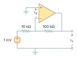
2. Find the gain  $v_o/v_s$  of the following circuit.
