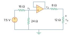
9. \*\*Determine the voltage gain  $v_o/v_i$  of the op amp circuit in the circuit below.
