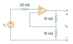
3. Calculate the voltage ratio  $v_o/v_s$  for the op amp circuit below.
