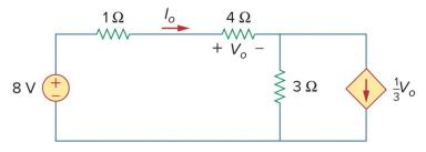
8. Apply the source transformation method to find  $i_x$  in the circuit below.
