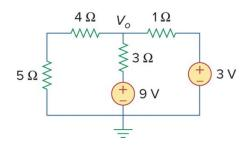
2. Use superposition to find  $v_o$  and  $i_o$  in the circuit below.
