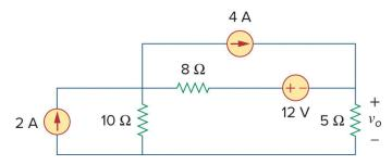
4. Using superposition, find  $V_{\rm o}$  in the following circuit.
